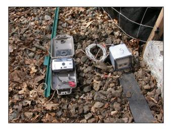
Photo 3. Modified Deercam<sup>®</sup> and infrared-triggered remote photography system prior to installation. Woodlot Alternatives, 2003.
