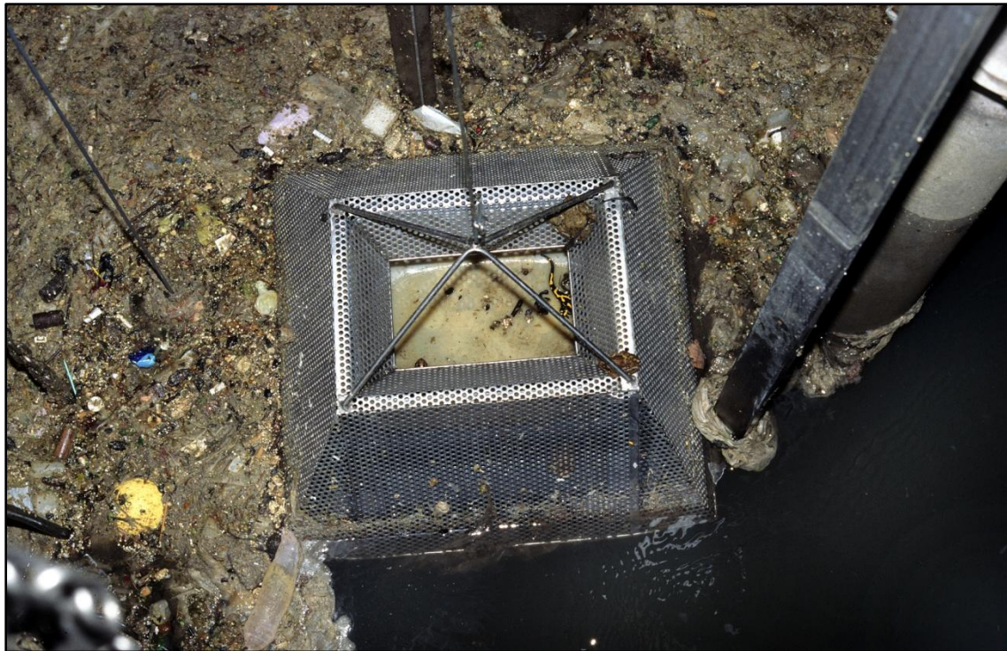
Figure 11. The floating bucket has a shape that does not allow animals to escape once they climb in. It is managed by a cable and pulley.
