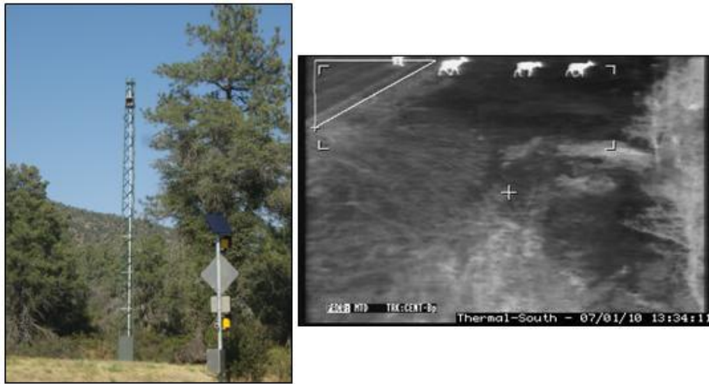
Figure 3. The tower-mounted infrared detection camera as part of the animal-activated detection system (AADS; left), and an infrared camera image of elk detected moving through the detection zone (right) after which radio signals activate motorist alert signage.
